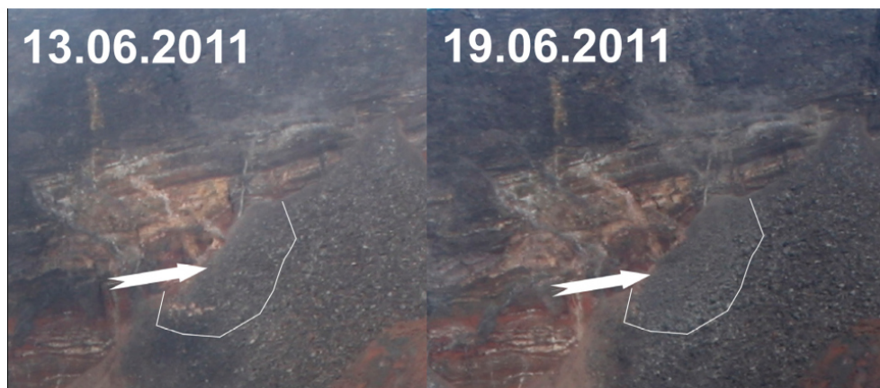
Figure 10. The white arrows show visually detectable surface changes (DoDs) in rock zone II between 13 June 2011 and 19 June 2011.
