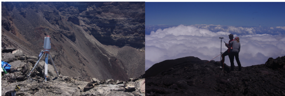
Figure 2. Riegl VZ4000 laser scanner located on the crater rim and dGNSS measurement of tie points (Riegl reflector) (own photographs captured during fieldwork in 2014).
