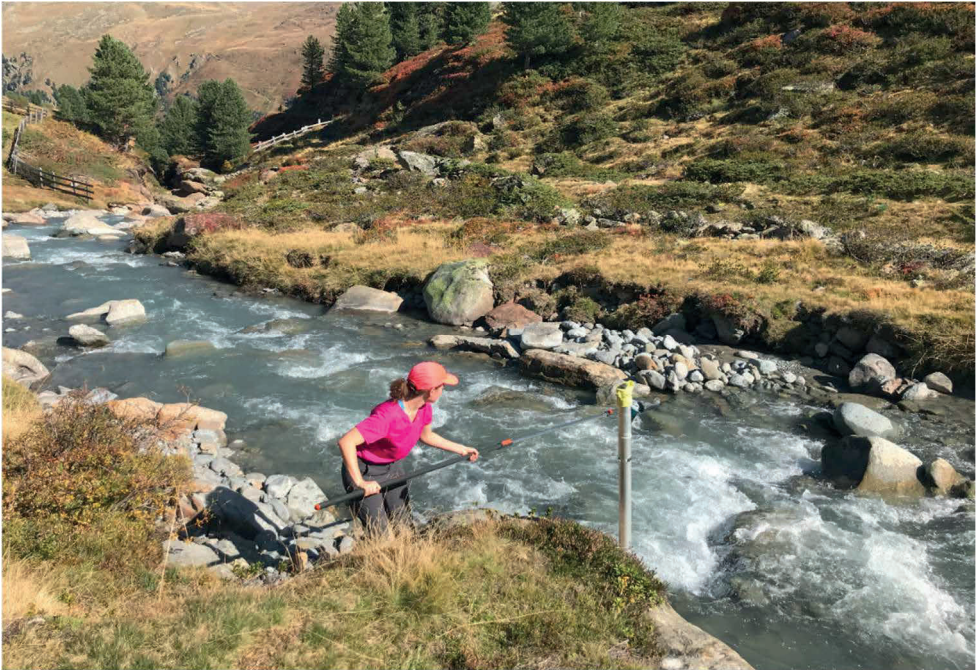
Figure 1: Water sampling for suspended sediment concentration measurement at Kauner Valley (Tyrol, Austria). Foto by: Kara, D.-E. 2023
